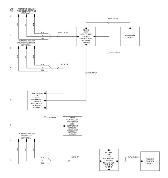
120V Air Con. & Cooler One-line Diagram
